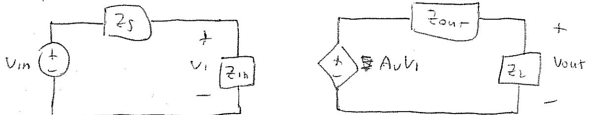
$$V_{out} = \frac{Z_L}{Z_{out} + Z_L} A_v V_i = \frac{Z_L}{Z_{out} + Z_L} \left( \frac{Z_{in}}{Z_S + Z_{in}} \right) V_{in} = V_{out}$$
