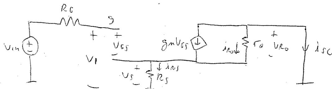
$$\text{NOTE: } i_{R_S} = -i_{SC} \Rightarrow V_S = -i_{SC} R_S$$
