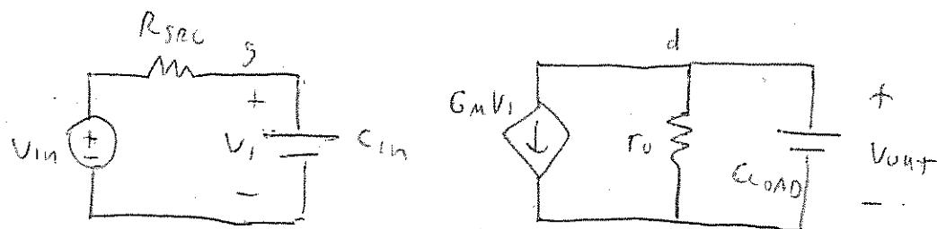
$$V_{out}(s) = -G_m V_1(s) \frac{1}{sC_{load}} \parallel r_o$$
