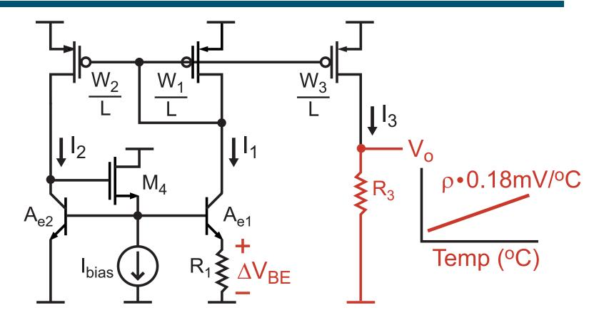
$$V_o = I_3 R_3 = \frac{W_3}{W_1} \left(\frac{\Delta V_{BE}}{R_1}\right) \frac{\beta}{\beta + 1} R_3 \approx \frac{W_3}{W_1} \frac{R_3}{R_1} \Delta V_{BE}$$
