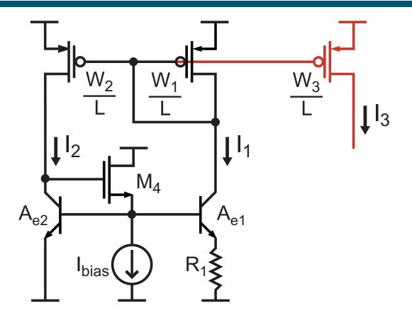
$$I_3 = \frac{W_3}{W_1} I_1 = \frac{W_3}{W_1} \left(\frac{\Delta V_{BE}}{R_1}\right) \frac{\beta}{\beta + 1}$$
