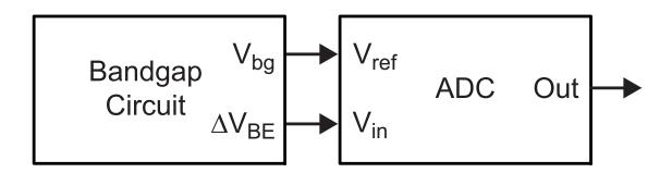
■ Recall that  $\Delta V_{BE}$  is a linear function of temperature
