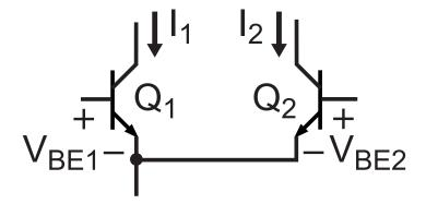
Subtraction of V<sub>BE</sub> voltages corresponds to division of collector currents
