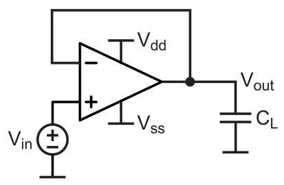
Consider the closed loop, unity gain configuration above with a sine wave input
