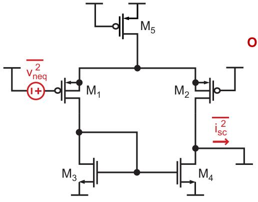
Output noise due to equivalent input-referred noise:
