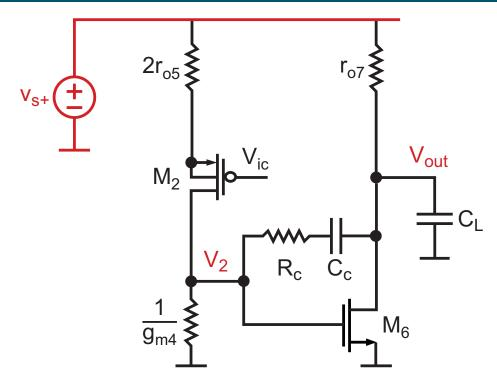
Calculation of impact of V<sub>s+</sub> on V<sub>out</sub>
