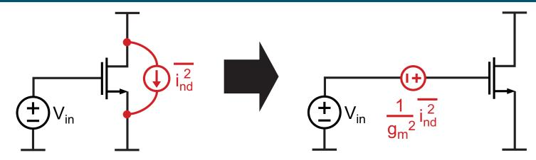
Transistor drain current noise:
