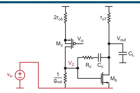
Calculation of impact of V<sub>s</sub> on V<sub>out</sub>
