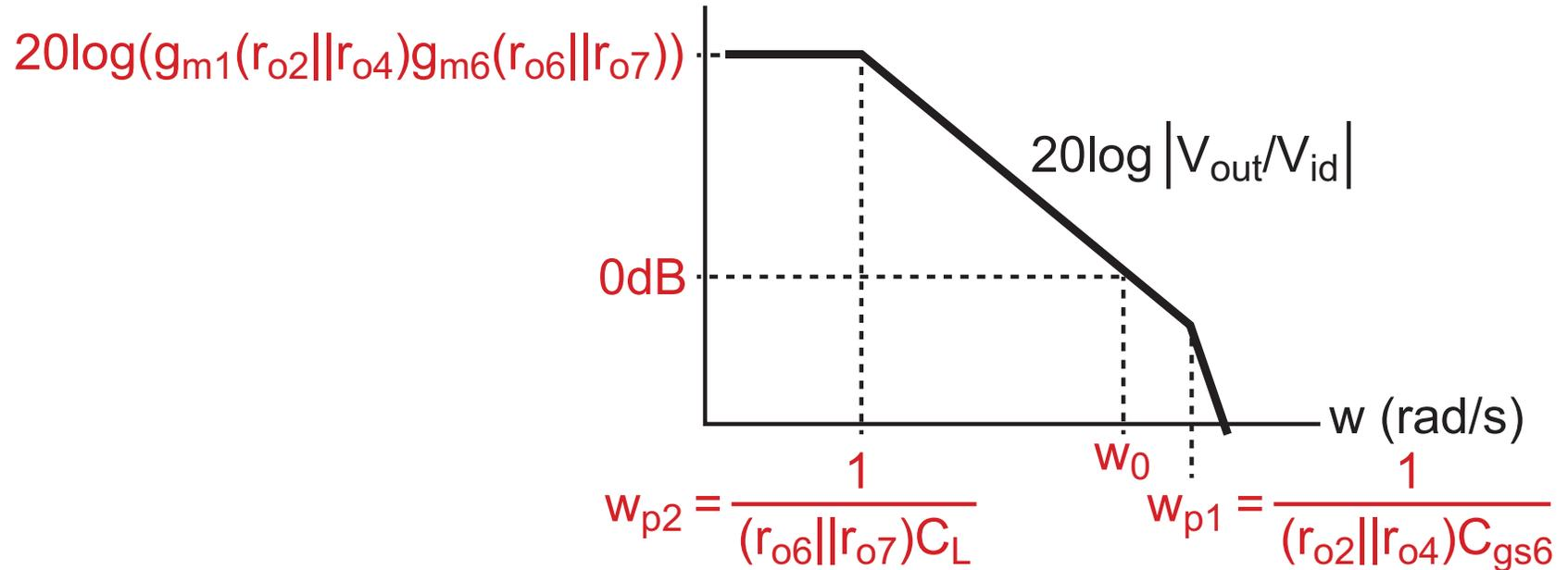
$$w_0 \approx \frac{g_{m1}(r_{o2}||r_{o4})g_{m6}}{C_L}$$
