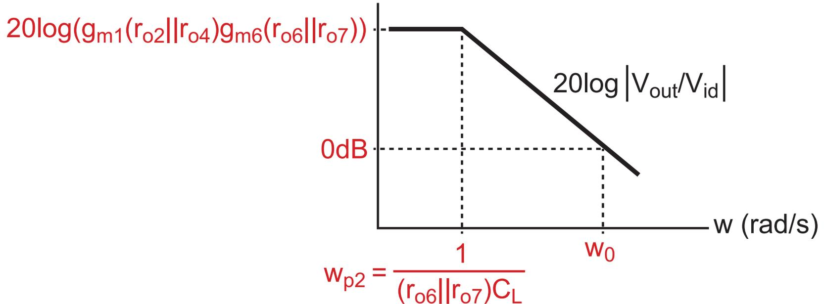
$$H(s) = \frac{K}{1 + s/w_{p2}} = \frac{g_{m1}(r_{o2}||r_{o4})g_{m6}(r_{o6}||r_{o7})}{1 + s(r_{o6}||r_{o7})C_L}$$
