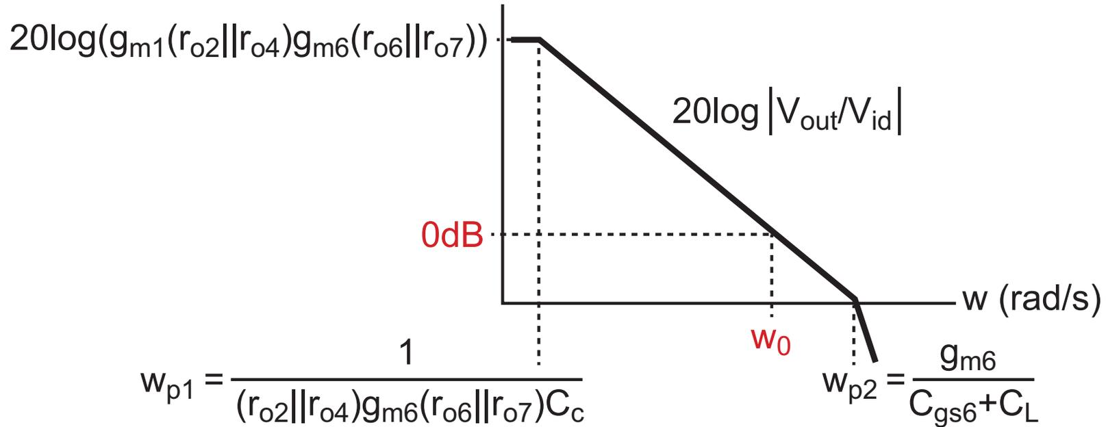
$$H(s) = \frac{K}{1 + s/w_{p1}} = \frac{g_{m1}(r_{o2}\parallel r_{o4})g_{m6}(r_{o6}\parallel r_{o7})}{1 + s(r_{o2}\parallel r_{o4})g_{m6}(r_{o6}\parallel r_{o7})C_c}$$
