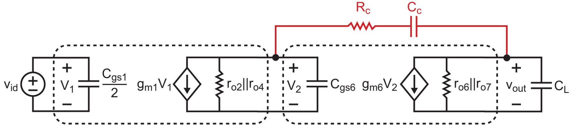
$$H(s) = \frac{v_{out}(s)}{v_{id}(s)} = \frac{K(1 + s/w_z)}{(1 + s/w_{p1})(1 + s/w_{p2})}$$
